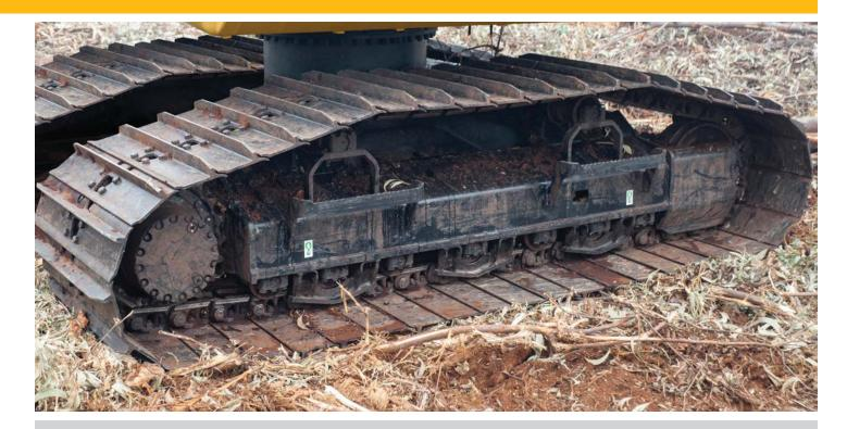
Caterpillar uses advanced engineering and software to analyze all structures, creating a durable, reliable machine for robust applications. More than 70 percent of the structural welds are robotic and achieve additional penetration over manual welds. These structural components and undercarriage are the backbone of the machine's durability.
